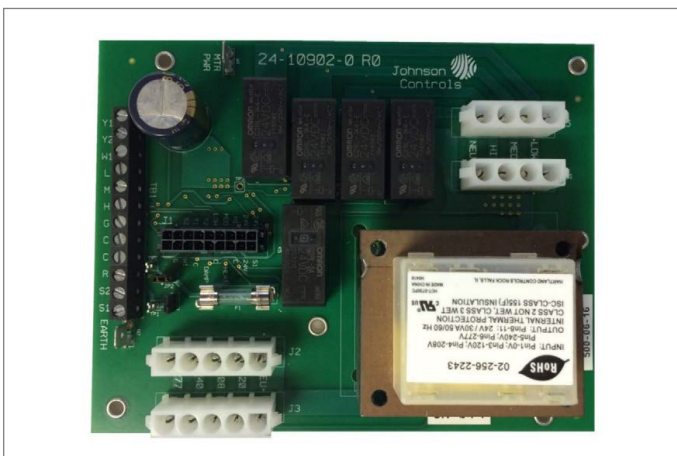
Figure 1 – Fan Relay Board (FRBii)
