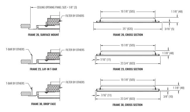
NOTES: Dimensions in parentheses are millimeters (mm). Illustrations shown are for 24"x24" panel size.
