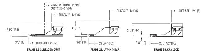
NOTES: Dimensions in parentheses are millimeters (mm). A 24"x24" panel with F23 or F29 is not available with a 20"x20" inlet size.
