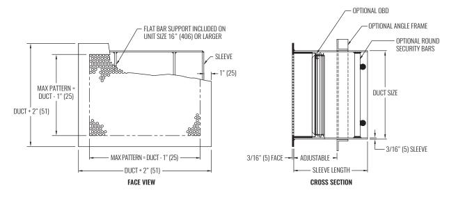
NOTES: Dimensions in parentheses are millimeters (mm). Recommended opening = duct size + 1/2". Optional angle frame or loose angles to be field welded for mounting.
