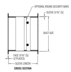
NOTES: Dimensions in parentheses are millimeters (mm). Recommended opening = duct size + 1/2". Optional angle frame or loose angles to be field welded for mounting.
