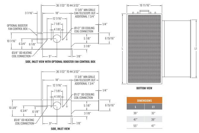
NOTES: Cooling/heating water pipe connections are copper 1/2" and 3/8" with wall thickness of 0.04". The maximum chilled/hot water circuit operating pressure is 150 psi.
