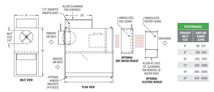
NOTES: Left-hand unit with electronic control enclosure shown; right-hand is available. Discharge requires flanged duct; connection by others. See table below for dimensional references.
