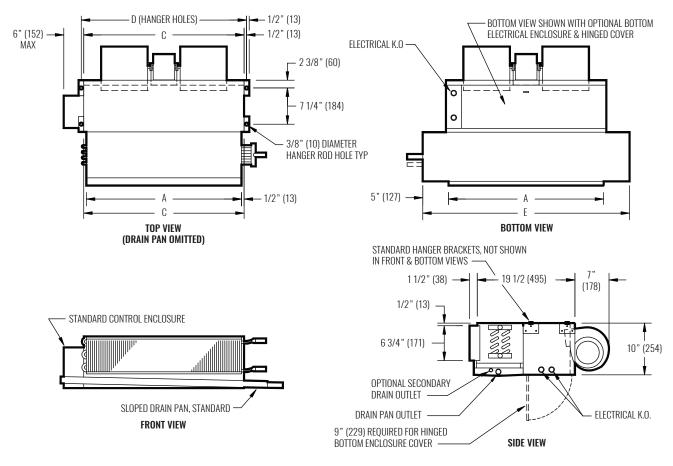
NOTE: Left hand coil shown, right hand is available. Provide access clearance for electrical enclosure per local and national electrical code requirements. Dimensions in parentheses are in millimeters (mm). See table below for dimensional references.
