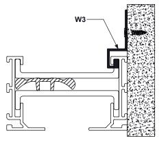
• USED WITH FRAME TYPE A OR D FOR INSTALLATION OF DFL PERPENDICULAR TO A WALL, WHERE FLANGE EDGE IS FLUSH AGAINST THE WALL. CANNOT BE USED WITH DFP PLENUM
