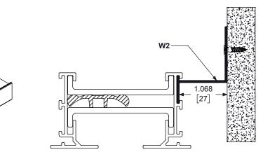
• USED WITH FRAME TYPE A, C, D, OR F FOR INSTALLATION OF DFL PERPENDICULAR TO A WALL WITH A REVEAL EFFECT BETWEEN THE FLANGE AND WALL
