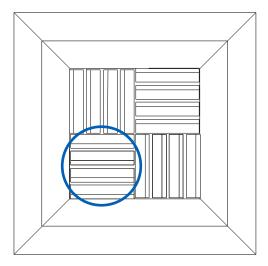
The area encircled represents one core. Each core represents one quarter section of the diffuser.
