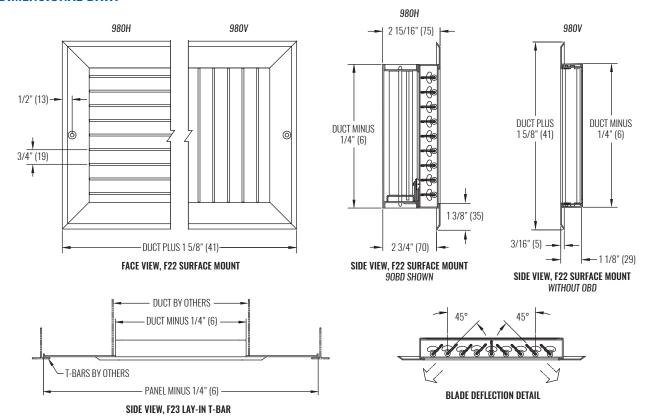
NOTE: Dimensions in parentheses are millimeters (mm).
