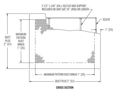
NOTE: Dimensions in parentheses are millimeters (mm).
