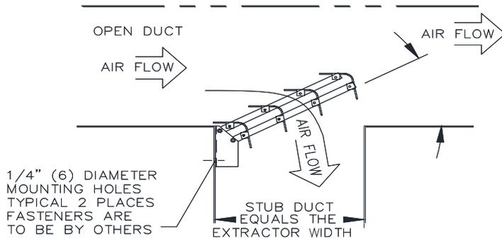
1/4" (6) DIAMETER MOUNTING HOLES TYPICAL 2 PLACES FASTENERS ARE TO BE BY OTHERS
