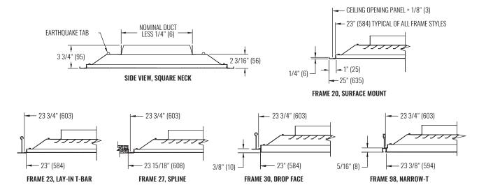
NOTES: Dimensions in parentheses are millimeters (mm). Illustrations shown are for 24"x24" panel size.
