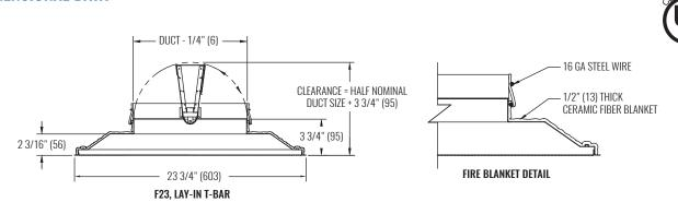
NOTES: Dimensions in parentheses are millimeters (mm). Illustrations shown are for 24"x24" panel size.
