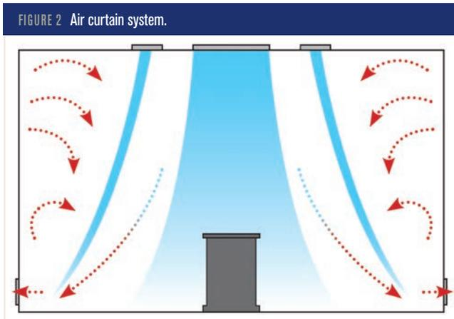
air outlet panels. Breaks between panels are dangerous and can provide a pathway for infectious particles to be induced into the supply airstream.
